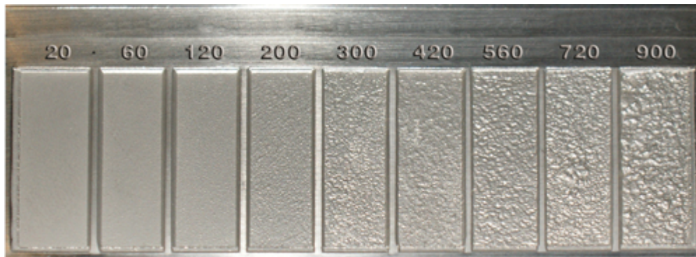
Figure 3—American Foundry Society's C-9 Microfinish Comparator (shows surface finishes from 20 RMS to 900 RMS)
